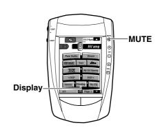
When using the remote controller, select AV Amp in the Home menu to display the operation menu. Then tap the down scroll button twice to display the third operation menu (Dim, Sleep, CH Sel, and +/-) or tap the down scroll button to display the next operation menu (Display).
